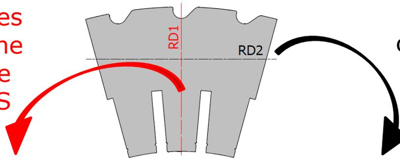
**-21%** of losses compared to the same machine made of NOES
